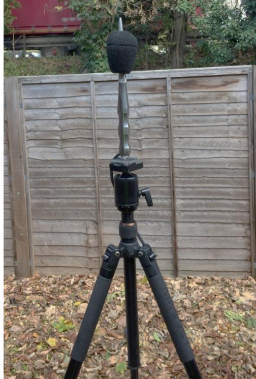
Plate 3.6 Typical noise monitoring equipment
